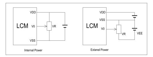
$V_{DD-}V_0$ : LCD Driving voltage VR: 10k~20k
